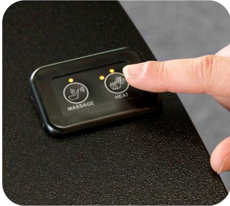
**Pressing the button the first time will start the heater at low power** and one light will come on. At this setting, it will take approximately 16.5 minutes to come to full heat **with an occupant in the chair**. Pressing the button a second time will take the heater to medium power (two lights on) and a third will take it to high (three lights on). To turn the heater off, press the button a fourth time and all the lights will be out.
